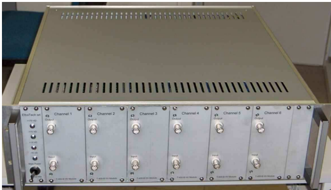
Front view of a 6 channels T-100 High Voltage Amplifier. Input and output connectors are available at the front panel.
